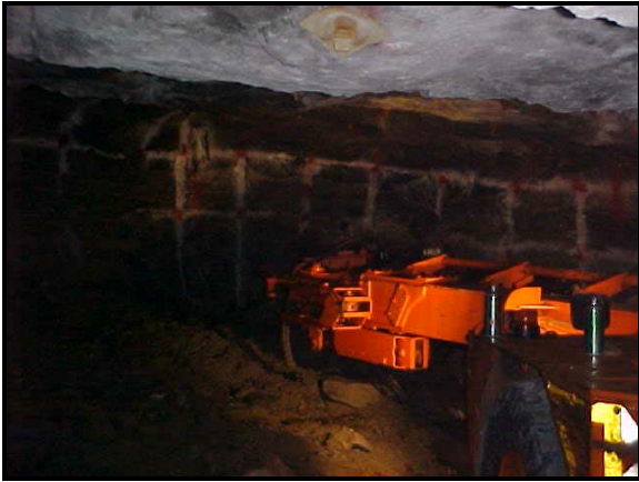
Drill rig drilling face blast holes
