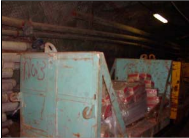
Material Cars modified for overhead crane
