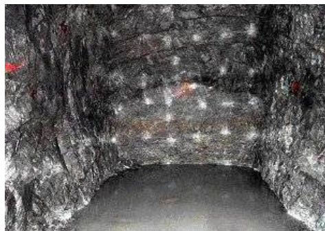
Fig 35. Clean break after blast with pumpable watergel, some barrels can be seen at lower left
