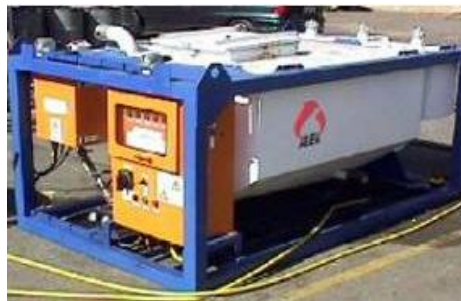
Fig 32. Emulsion charging unit U 117E
