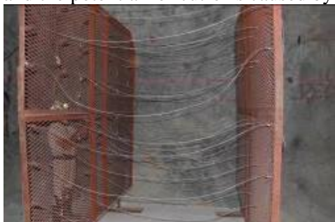
Figure 18. Shock tube timing test rig, side views
