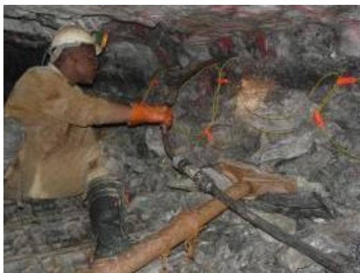
Figure 42: Charging-up in progress
