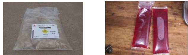
Figure 40: Bagged emulsion and sachet of the gassing agent
