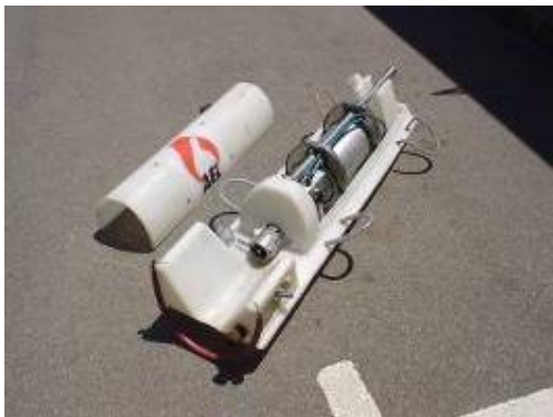
Figure 38a: The US05 pump disassembled
