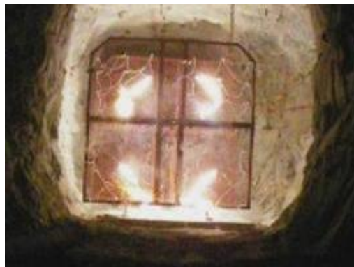
Figure 19. Photograph of the shock tube blast in progress on the test rig
