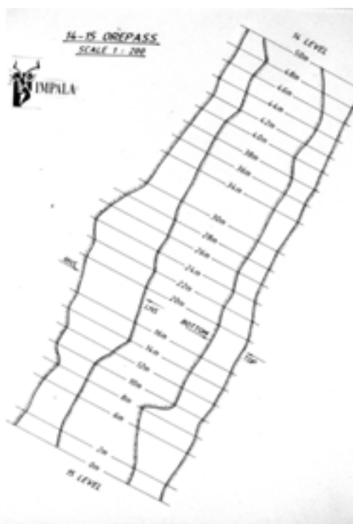
Figure 1 – sections through ore pass
