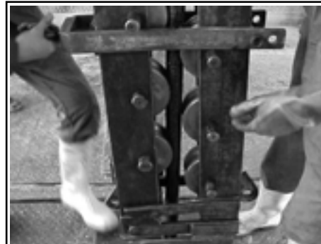
Figure 13: Device to iron out kinks in the rope
