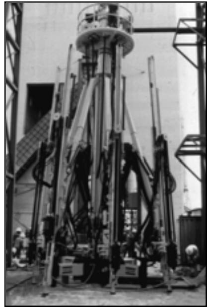
Figure 24: Atlas Copco Jumbo drill rig
