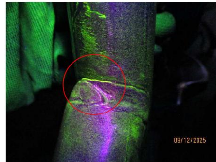
Fig 16: Chairlift No: 46 Cold lap indications noted.
