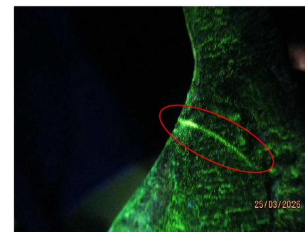
Fig 9: Stretcher Carrier No: SI/141 Crack like indications noted.
