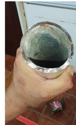
Figure 2: Rust and Water Ingress at Crack Origin
